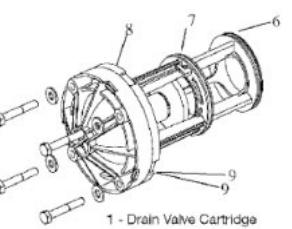
1 - Drain Valve Cartridge
