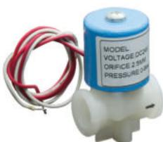
Two-way solenoid valve NC direct acting; Body material plastic; Seals in EPDM; Spring in SS304; Range water temperature = 4°C ÷ 120°C; Range ambient temperature = -10°C ÷ +40°C; Range pressure = 0 ÷ 8 bar; Class protection IP65; Connections ¼" NPT; Orifice diameter 2,5 mm;
