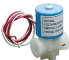
Two-way solenoid valve NC direct acting; Body material plastic; Seals in EPDM; Spring in SS304; Range water temperature = 4°C ÷ 120°C; Range ambient temperature = -10°C ÷ +40°C; Range pressure = 0 ÷ 8 bar; Class protection IP65; Connections 1/4" NPT; Orifice diameter 2,5 mm;
