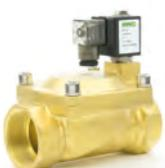
Two-way solenoid valve NC indirect acting; Body material brass; Seals in EPDM; Range water temperature = 4°C ÷ 120°C; Class protection IP65; G thread connections;
