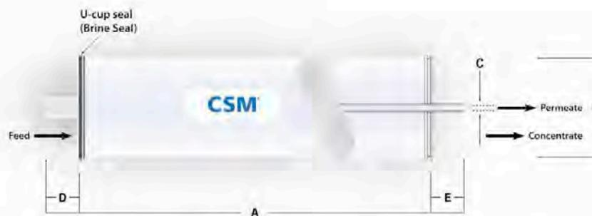
1. Each membrane element comes with one brine seal, one interconnector (coupler) and four o-rings.
