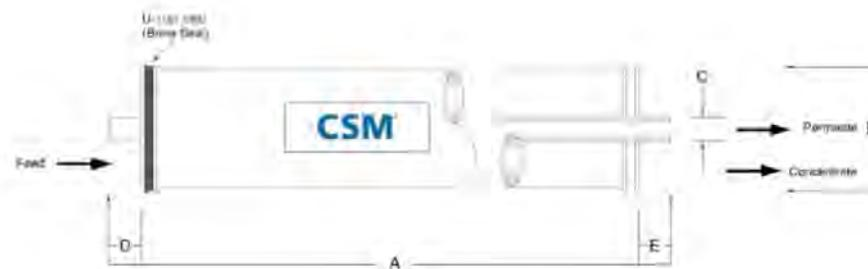
1. Each membrane element supplied with one brine seal, one interconnector (coupler) and four o-rings.
