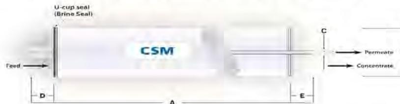
1. Each membrane element supplied with one brine seal, one interconnector (coupler) and four o-rings.
