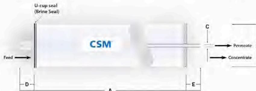
1. Each membrane element supplied with one brine seal, one interconnector (coupler) and four o-rings.
