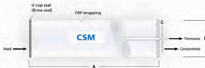
1. Each membrane element supplied with one brine seal, one interconnector (coupler) and four o-rings.
