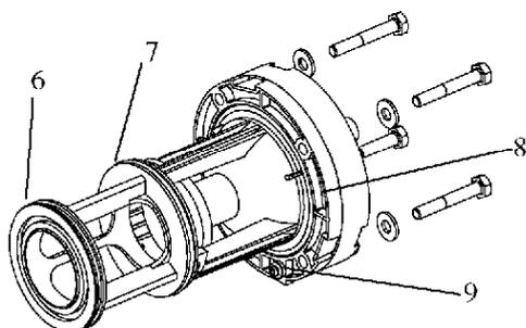
3 - No Hard Water Bypass Valve Cartridge
