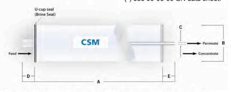
1. Each membrane element comes with one brine seal, one interconnector (coupler) and four o-rings.
