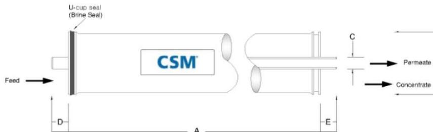
1. Each membrane element supplied with one brine seal, one interconnector (coupler) and four o-rings.
