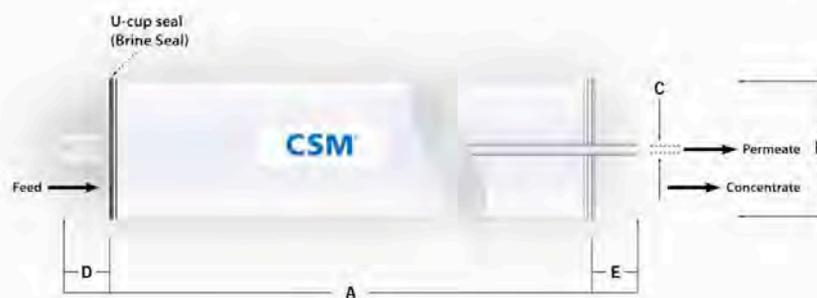
1. Each membrane element supplied with one brine seal, one interconnector (coupler) and four o-rings.
