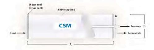
Each membrane element supplied with one brine seal, one interconnector (coupler) and four o-rings.
