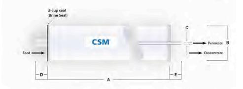
Each membrane element supplied with one brine seal, one interconnector (coupler) and four o-rings.
