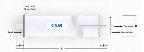
1. Each membrane element supplied with one brine seal, one interconnector (coupler) and four o-rings. 2. All RE2540 elements fit nominal 2.5 inch (64 mm) I.D. pressure vessels.
