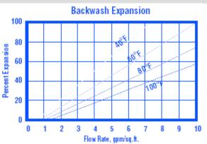
**Backwash:** After each cycle the resin bed should be backwashed at a rate that expands the bed 25 to 50 percent. That will remove any foreign matter and reclassify the bed. The graph above shows the expansion characteristics of Pure PC002 in the sodium form.
