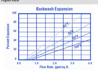
**Backwash:** After each cycle the resin bed should be backwashed at a rate that expands the bed 50 to 75 percent. That will remove any foreign matter and reclassify the bed. The graph above shows the expansion characteristics of Pure PA103.
